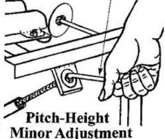
During operation, if the height adjusting handle tends to "walk" (not stay in the same position), then the locknuts underneath the height adjusting bracket can be "locked" against the bracket itself, but be sure to "unlock" the lock nuts before making further adjustments and then retighten afterwards.
